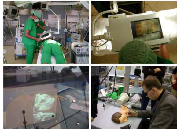
Figure 2.14: Example of a screen-based AR display using a see-through LCD panel – The AR window (upper-left and -right) [Sch02]. Courtesy: ZGDV, Schwald. Example of a mirror-based AR display using optical see-through beam splitters (lower-left and -right). Courtesy: Fraunhofer IMK (www.arsys-tricoder.de).
