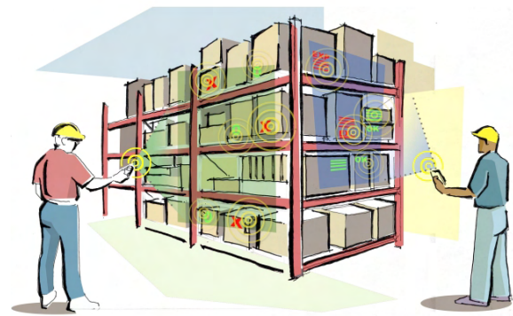
Figure 5.2: Warehouse scenario using RFIG (Ras04). A user directs a handheld projector at tagged inventory, with communication mediated by two channels -- RF and photo-sensing on the tags. The user sees a projection of the retrieved tag information collocated with the physical objects, and performs a desktop-like interaction with the projection. A second user performs similar operations, without conflict in the interaction because the projector beams do not overlap.
