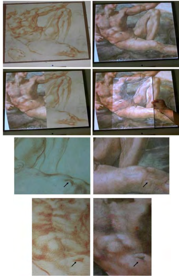
Figure 4.29: Results of color correction process with a single projector on real drawing: (a) Real drawing (64x48cm) under environment light. (b) Output image emitted onto drawing. (c) Partially augmented drawing. (d) Output image on a white piece of paper. (e-h) Close-ups. While the upper body part coincides in drawing and painting, Michelangelo modified the lower body part. The arrows indicate the displaced knee and belly sections. They point at the same spot on the drawing.
