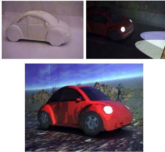
Figure 4.8: (Top-left) The diorama of a car and approximate background. (Bottom) A cartoon-like environment created by image projection in which the car appears to move (Top-right) A night-time simulation using virtual headlights.
