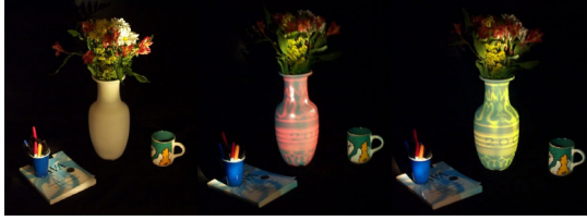
Figure 4.2: (Left) The underlying physical object is a white diffuse vase. (Middle and right) View-dependent effects, such as specular highlights, can be generated by tracking the user's location and projecting images on the vase.
