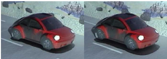
Figure 4.10: Vertical displacement by shifting the background and shadows. These two pictures are taken from the same camera position, so the car in both images is at the same location. Note the change in position of the virtual shadows and the parallax for the edge between ground and backdrop.
