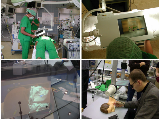
Figure 2.7: Example of a screen-based AR display using a see-through LCD panel – The AR window (upper-left and -right) 105 . Courtesy: ZGDV, Schwald. Example of a mirror-based AR display using optical see-through beam splitters (lower-left and -right). Courtesy: Fraunhofer IMK (www.arsys-tricorder.de).
