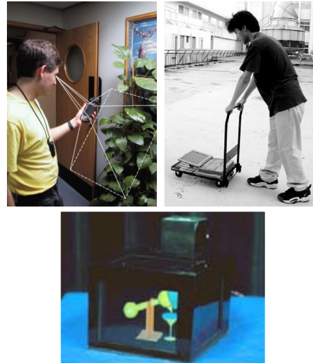
Figure 2.18: Example of a hand-held PDA-based AR display 82 (upper-left). Courtesy: AT&T, Newman, Ingram, and Hopper. The Virtual Glassboat 109 (upper-right). Courtesy: Siio. Example of an object-oriented Display – MEDIA3 54 (bottom). Courtesy: Kawakami, Inami, Sekiguchi, Yanagida, Maeda, and Tachi.
