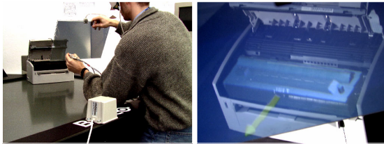
Figure 2.19: The Transflective Pad 8 – a hand-held mirror beam-splitter in combination with a large rear-projection screen.
