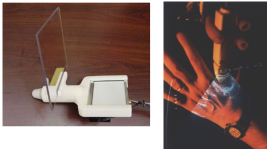
Figure 2.17: Example of a hand-held mirror display - The Sonic Flashlight 112 . Courtesy: Stetton, Chib, Hildebrand, and Bursee.
